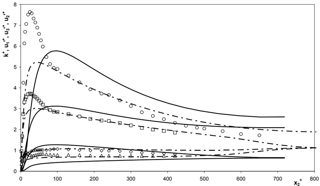
Figure 10. Comparison between the predicted and the measured profiles of normalized turbulent kinetic energy and Reynolds normal stresses for fully-developed turbulent pipe flow of 0.20% XG fluid at  $Re=39000$  in wall coordinates:  $\circ$   $k^+$  data of Escudier *et al.* (1999);  $\square$   $u_1^{+}$ ,  $\diamond$   $u_3^{+}$ ,  $\Delta$   $u_2^{+}$  data of Resende *et al.* (2006); — Present model; - - Resende *et al.* (2006).
