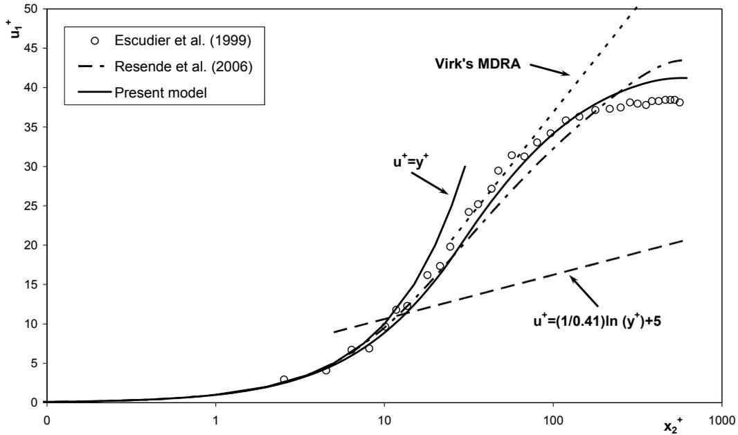
Figure 3. Comparison between the predicted and measured mean velocity profile for fully-developed pipe turbulent flow with the 0.125% PAA solution at  $Re=42900$  in wall coordinates.
