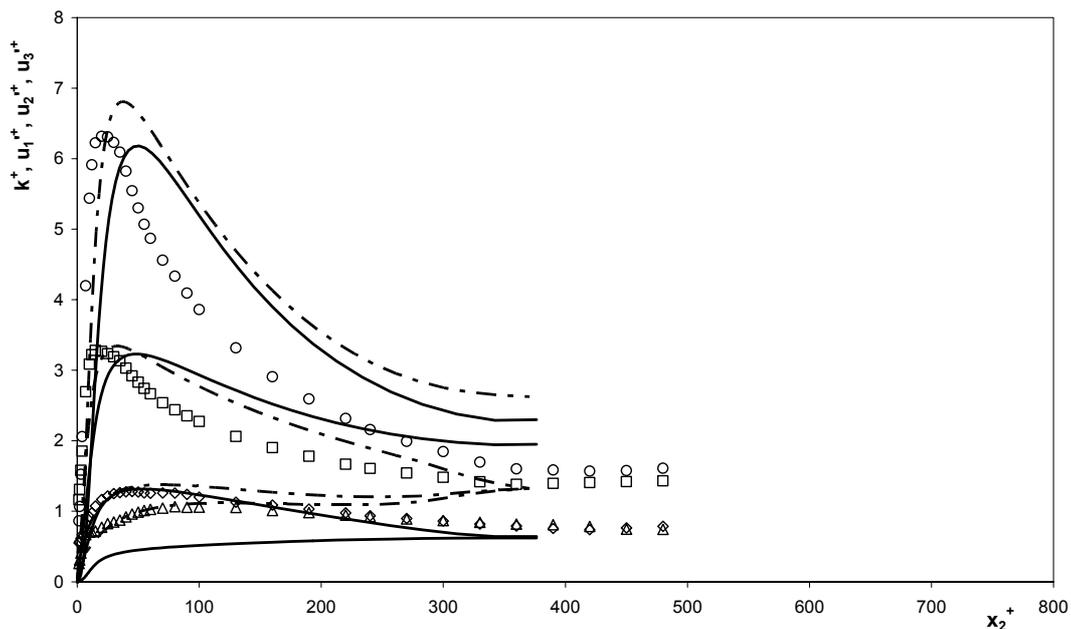
Figure 6. Comparison between the predicted and the measured profiles of normalized turbulent kinetic energy and Reynolds normal stresses for fully-developed turbulent pipe flow of 0.25% CMC fluid at  $Re=16600$  in wall coordinates:  $\circ$   $k^+$  data of Escudier *et al.* (1999);  $\square$   $u_1^{+}$ ,  $\diamond$   $u_3^{+}$ ,  $\Delta$   $u_2^{+}$  data of Resende *et al.* (2006); — Present model; — - Resende *et al.* (2006).
