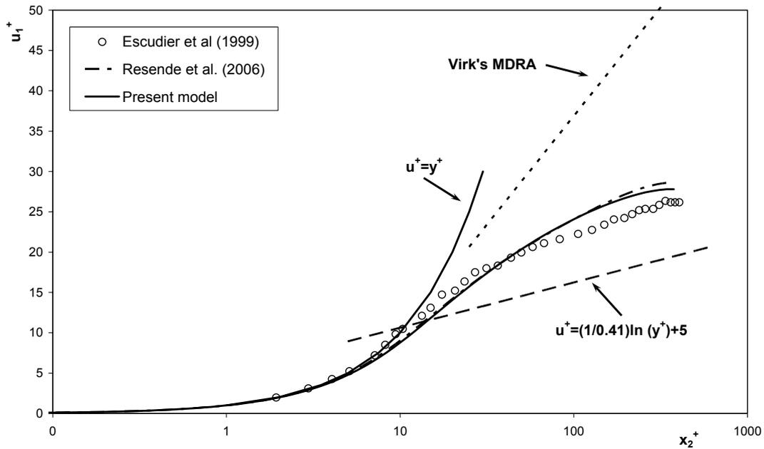
Figure 5. Comparison between the predicted and measured mean velocity profile for fully-developed pipe turbulent flow with the 0.25% CMC solution at  $Re=16600$  in wall coordinates.
