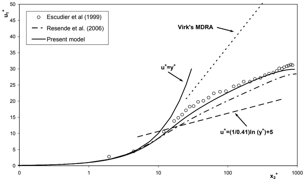
Figure 7. Comparison between the predicted and measured mean velocity profile for fully-developed pipe turbulent flow with the 0.09% / 0.09% CMC / XG solution at Re=45300 in wall coordinates.
