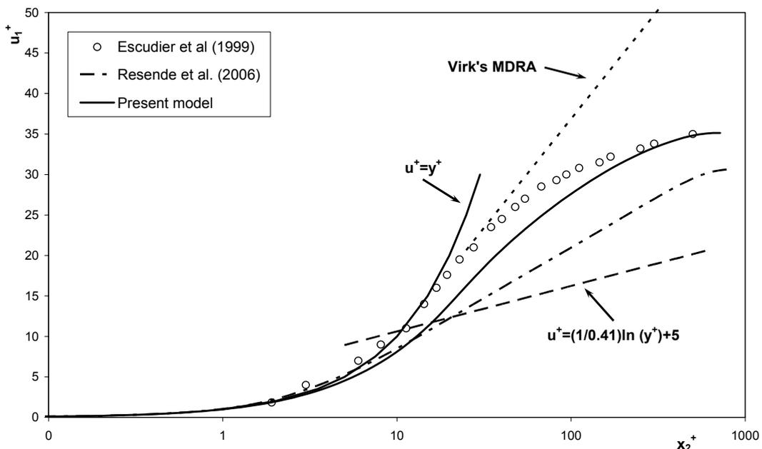
Figure 8. Comparison between the predicted and measured mean velocity profile for fully-developed pipe turbulent flow with the 0.2% XG solution at Re=3900 in wall coordinates.
