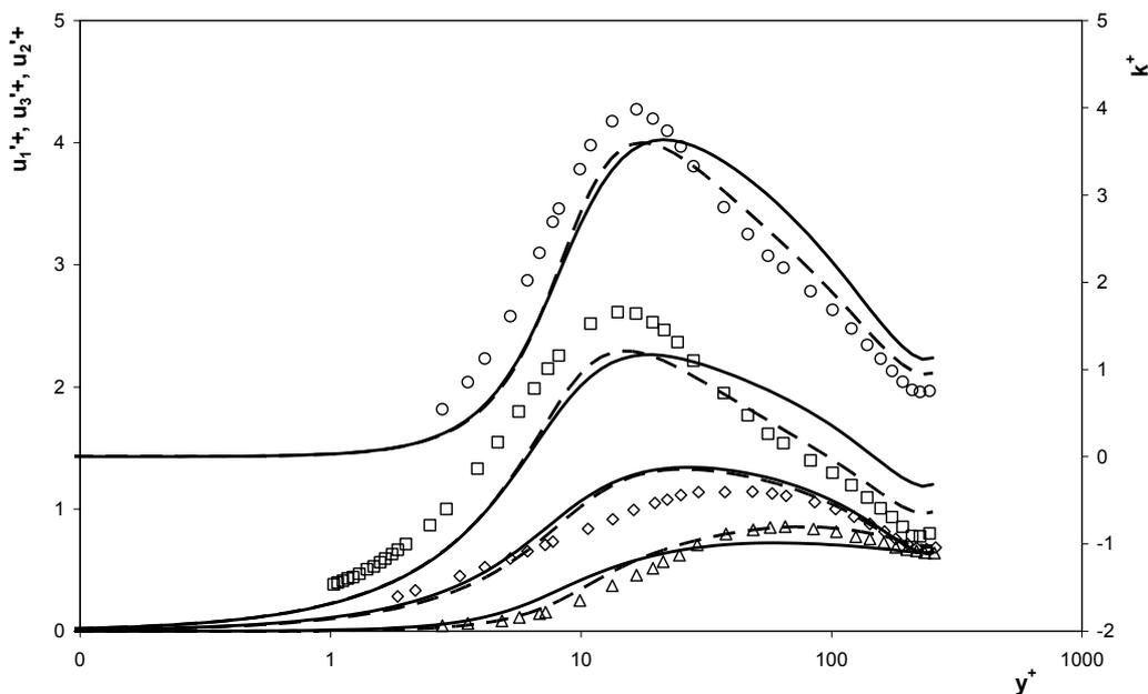
Figure 2. Comparison between the predicted and the measured profiles of normalized turbulent kinetic energy and Reynolds normal stresses for fully-developed turbulent pipe flow of Newtonian fluid at  $Re=7430$  in wall coordinates:  $\circ$   $k^+$ ,  $\square$   $u_1'^2$ ,  $\diamond$   $u_3'^2$ ,  $\Delta$   $u_2'^2$  data of Durst *et al.* (1995); — Present model; - - Lai and So model (1990).
